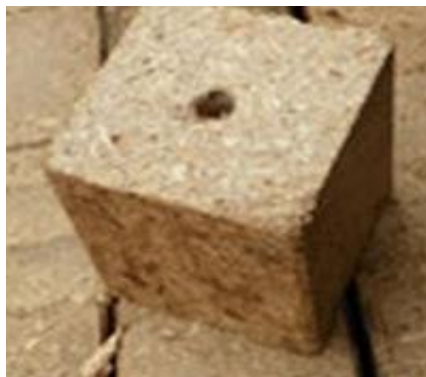
Figure (3) shows the recycling of wood waste to produce wooden blocks suitable for models of design ideas
